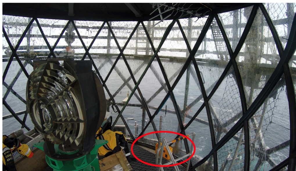
Figure 9. Yellow logger (data acquisition, storage, and communication) box in lantern room. Steel framework of helideck is visible outside.
