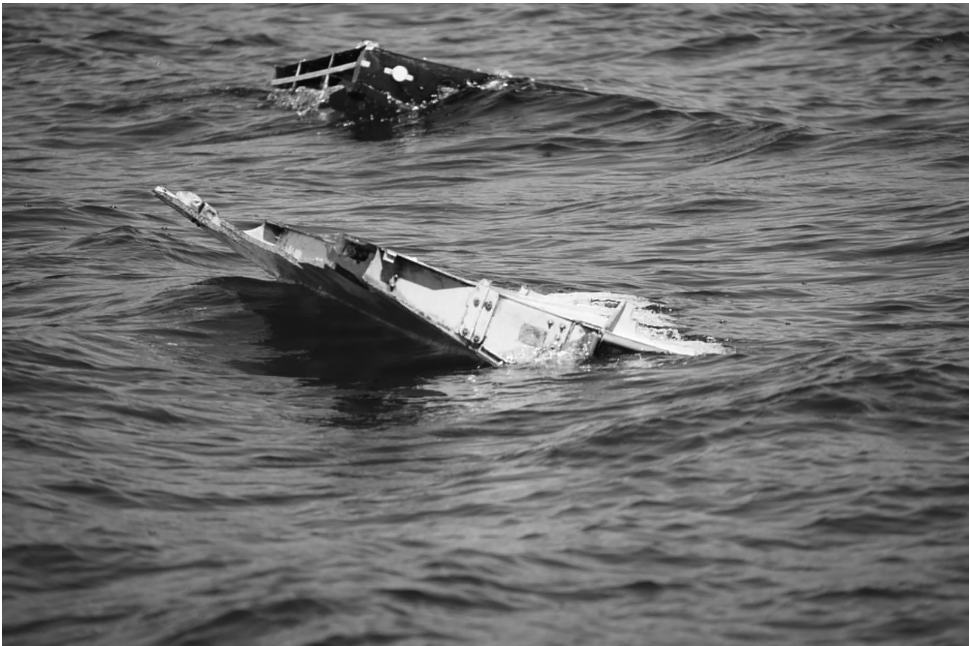
Figure 29.6 Actual and replica flaperons dropped into the field test area of Storm Bay, Tasmania, to assist in drift modeling simulations. Courtesy of Commonwealth Scientific and Industrial Research Organisation (CSIRO).
