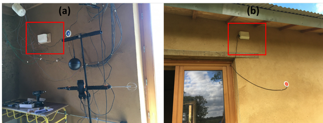
Figure 3. Indoor (a) and outdoor air quality (b) stations.
