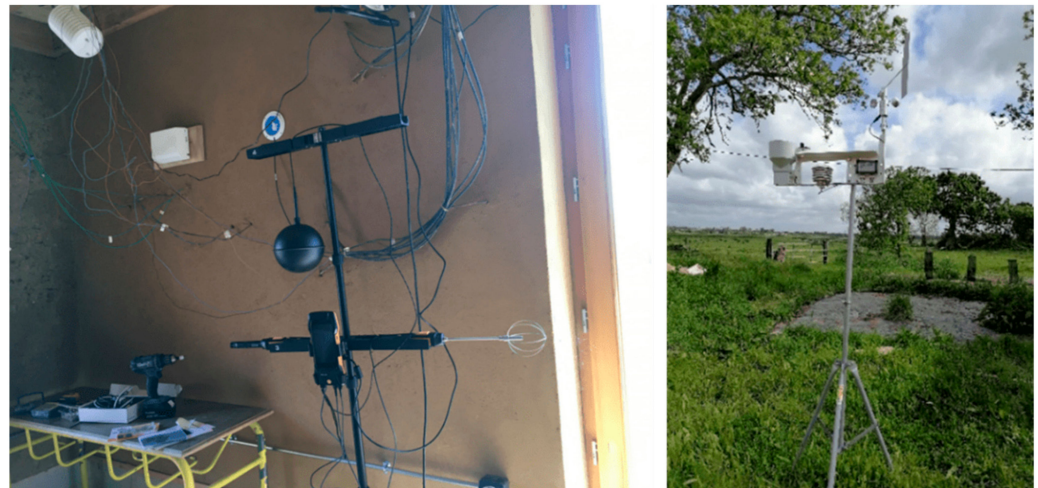
Figure 4. Monitoring of temperature and relative humidity inside and outside the prototype building.
