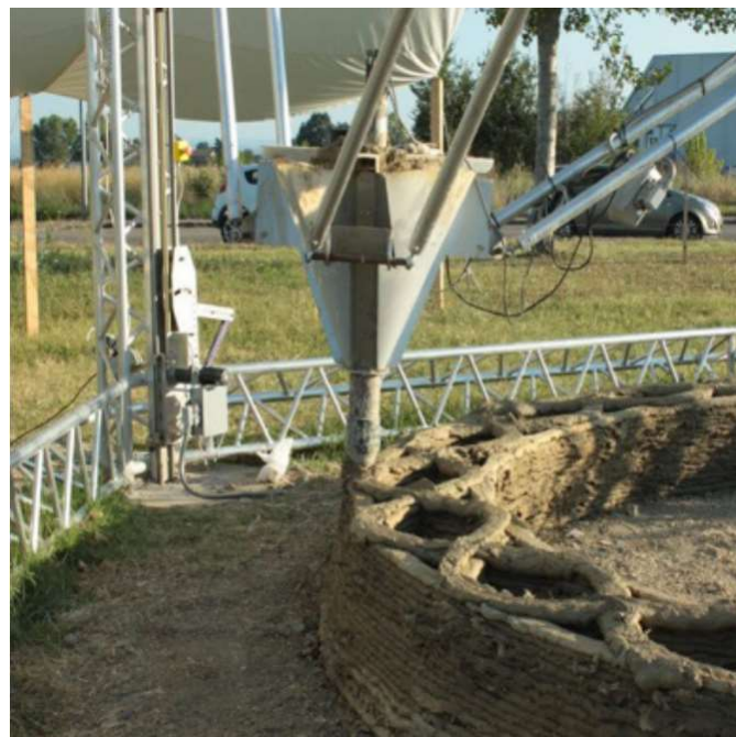
Figure 4. Screw pump extruder by WASP
