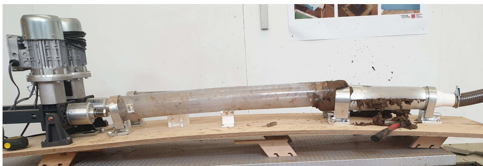
Figure 12. Buckling of the plywood platform due to accumulated pressures on nutrig points
