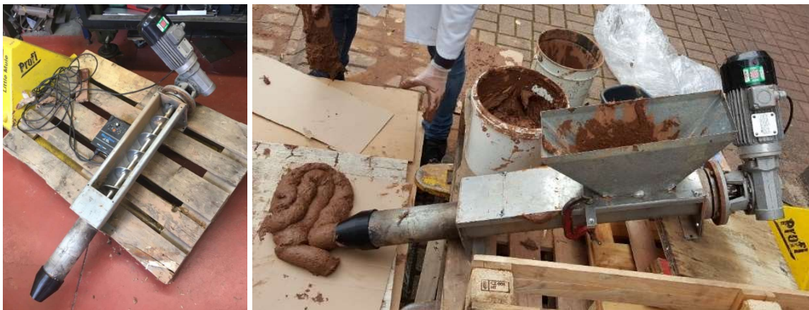
Figure 6. The prototype of the bespoke screw pump.
