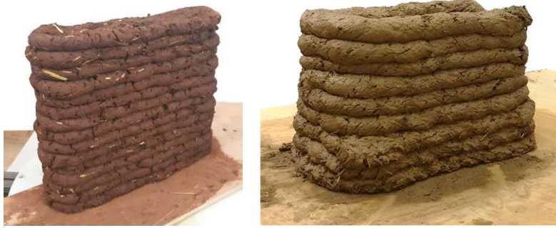
Figure 21. Prototypes showing the longitudinal deformation due to accumulative weight of layers (lower water content to left, higher water content to the right).
