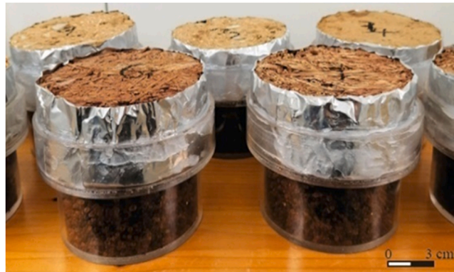
Fig. 10. Experimental water vapor permeability test.
