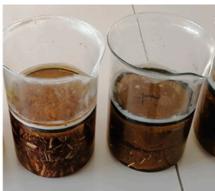
Step 1: Immersion of samples in non-wetting oil
