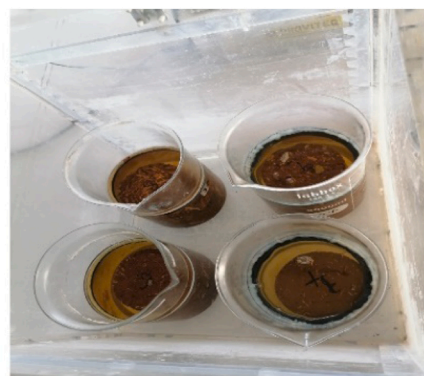
Step 2: Saturation under vacuum
