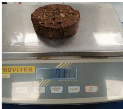
Step 3: Weighting of saturated sample in air
