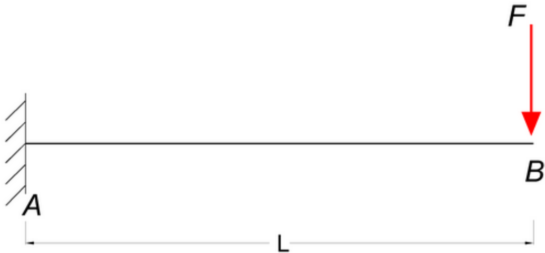
Figure 36: Cantilever beam schematic, point load
