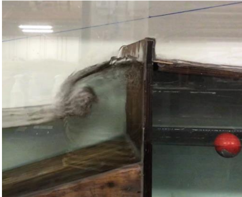
(a) 0.40 Hz – wave reflected by wall – no overtopping
