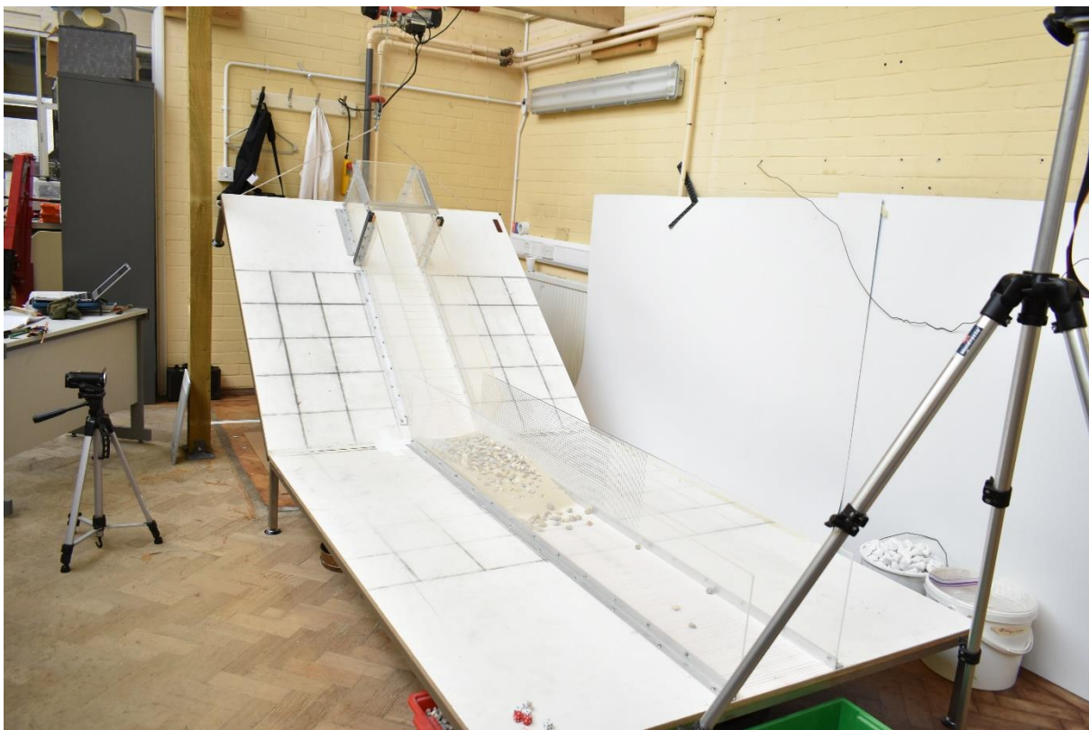
Figure 1: An image showing a view of the experiment setup along with the camera which records the side view of the flow and deposit.
