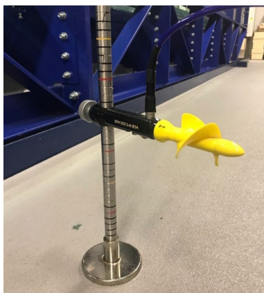
Figure 6: Valeport impeller used to measure the current speed.
