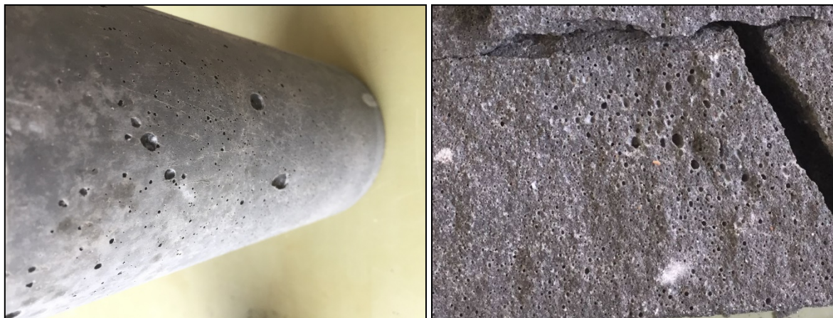
Figure 28: (left) - Bubbles possibly a result of poor compaction Figure 29: (right) - Entrained air throughout samples
