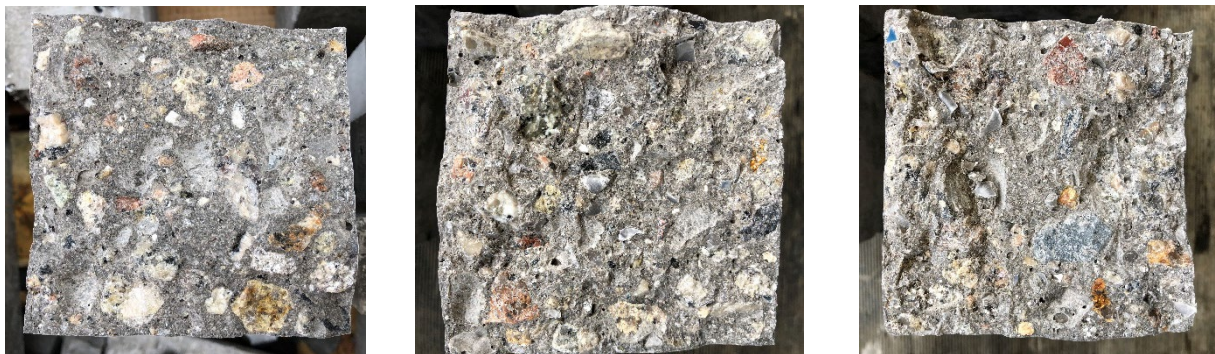
Figure 19: Concrete beam samples split open after flexural strength testing
