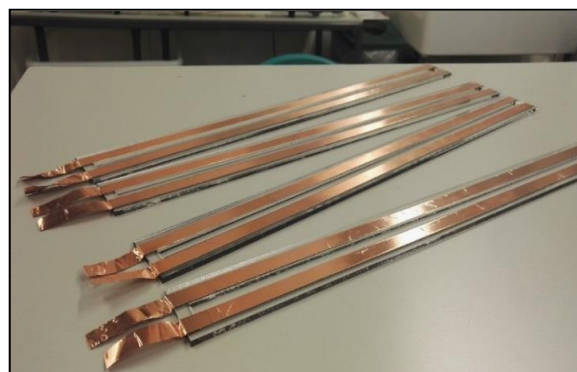
Figure 8: Wave gauges with copper tape attached
