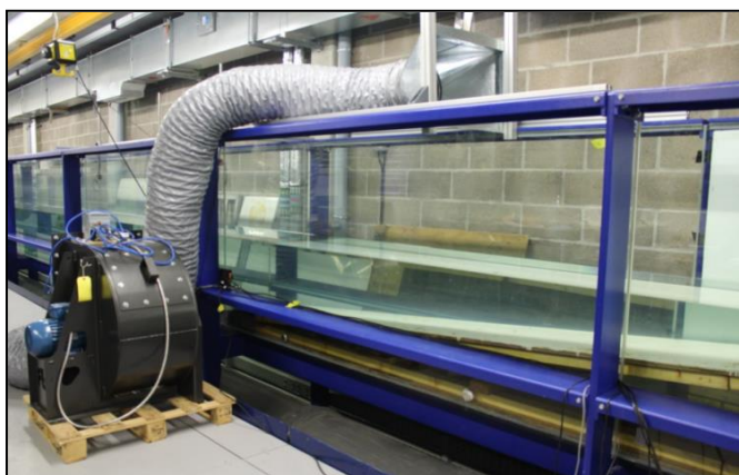
Figure 11: Wind generator set up
