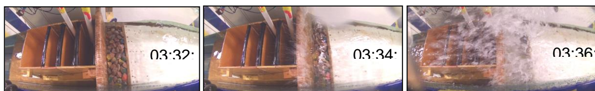
Figure 25: 0.7Hz wave with 4m/s wind showing significant splash overtopping with added time stamp
