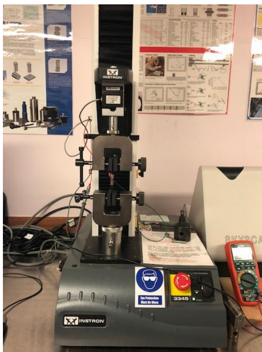
Figure 2: Instron 3345 used for tensile testing tube shaped sensors.
