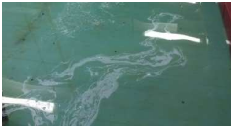
Figure 2 - Seeding material being added to the Basin
