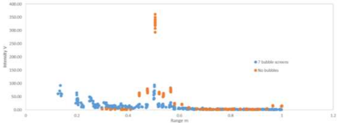
Figure 4.6: VA500 amplitude returns and ranges for a bubble free water column (orange) and a water column with 7 bubble screens (blue) at 6cm separation. Returns from individual bubble screens can be distinguished. The target return is considerably lower in amplitude in the presence of bubbles, with some returns lower in amplitude than the returns off the initial bubble layers.
