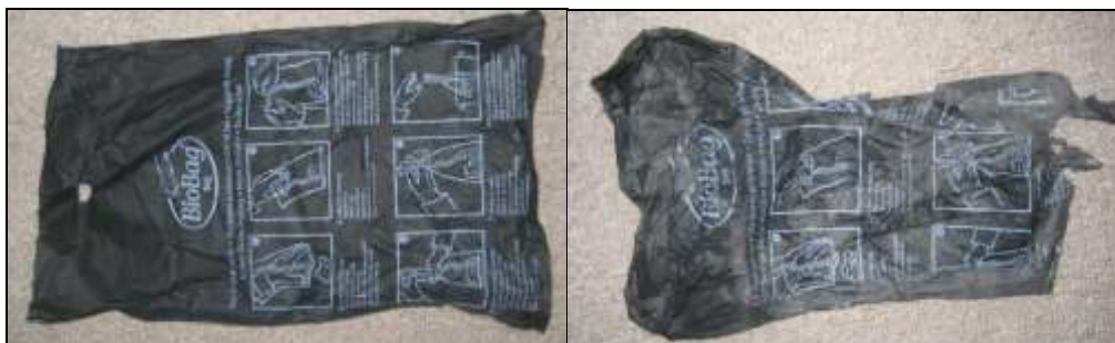
Fig 2.22 Bio bag before and after degradation buried in mud
