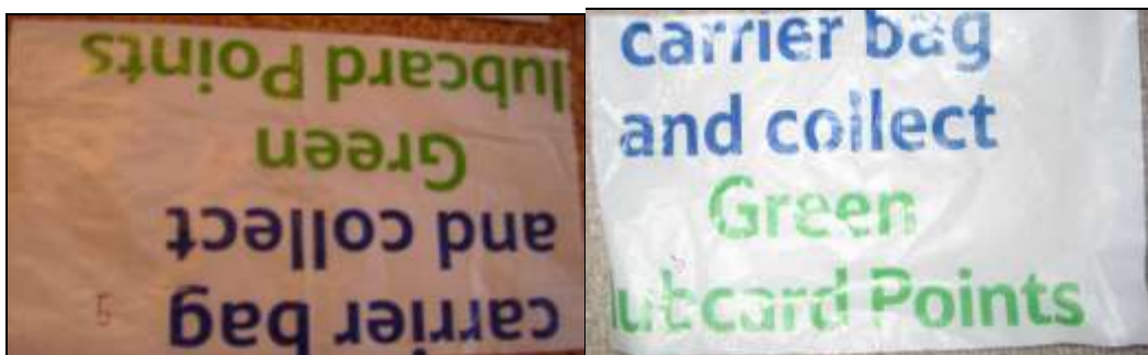
Fig 2.21 Tesco samples before and after degradation in dark salt water
