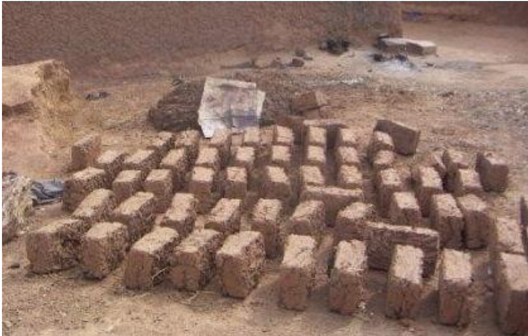
Figure 5.17: Curing of adobe blocks
