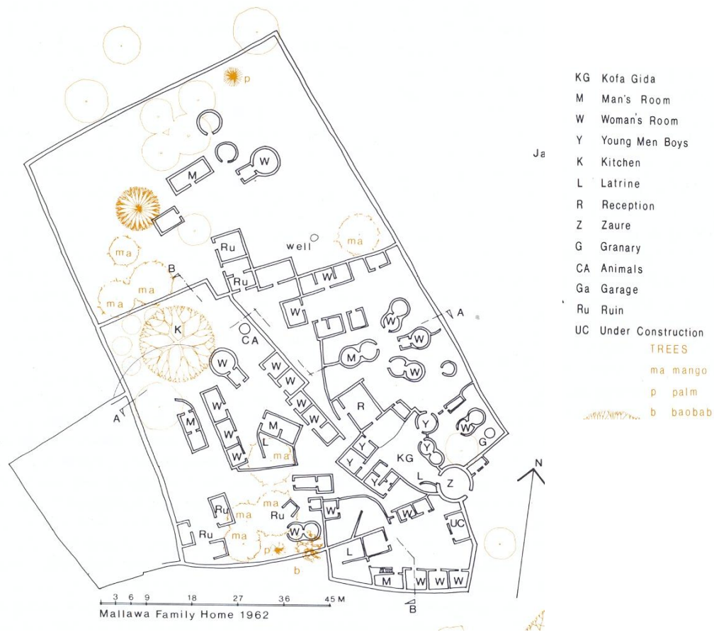
Figure 5.4: A layout plan of a traditional Hausa compound in Zaria City as recorded by Moughtin (1985:62)
