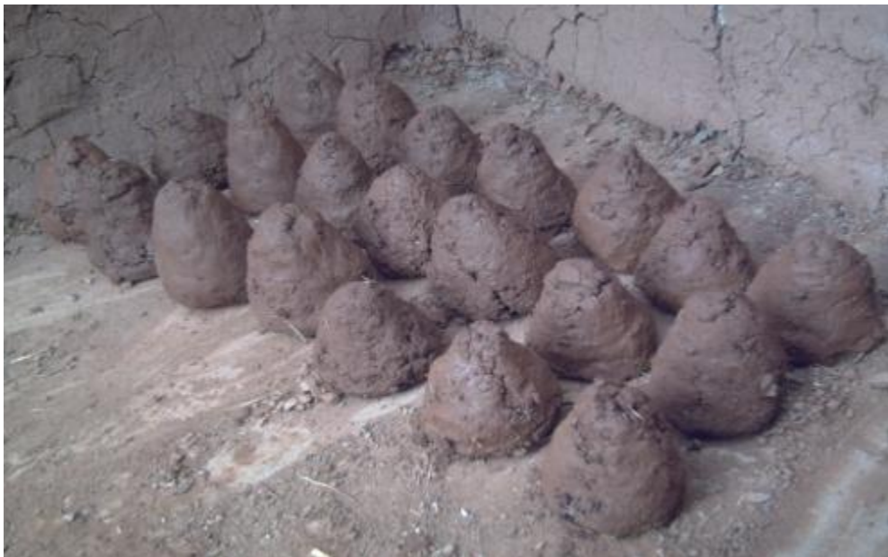
Figure 5.9: A freshly moulded tubali brick. The bricks were moulded by the author during the 'Cob Week' at the University of Plymouth in 2007
