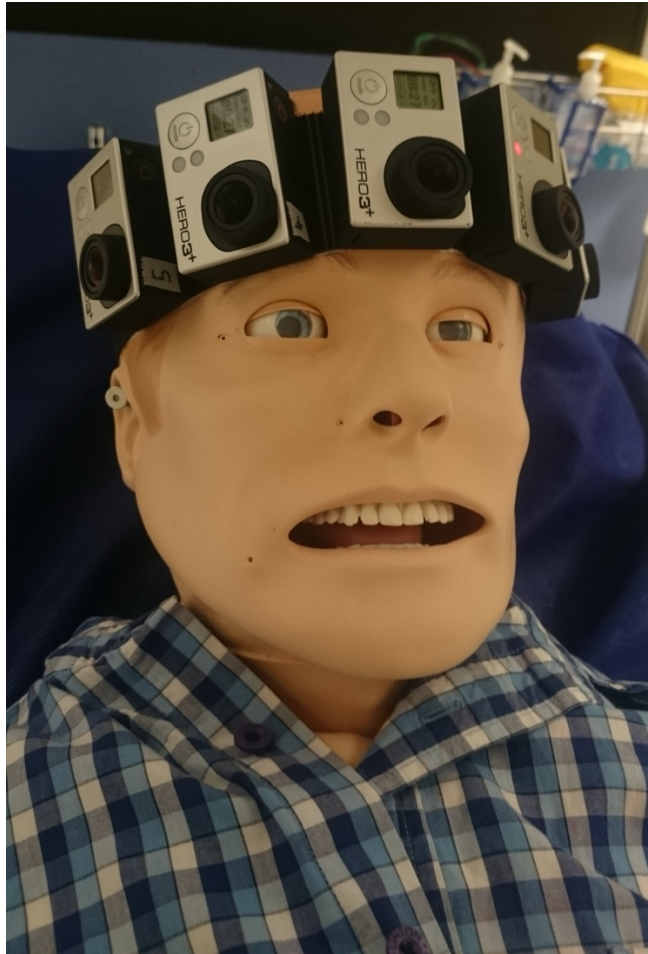
Figure 15 A pre-dedicated 360-degree camera rig on the manikin's head for perspective simulation scenario filming
