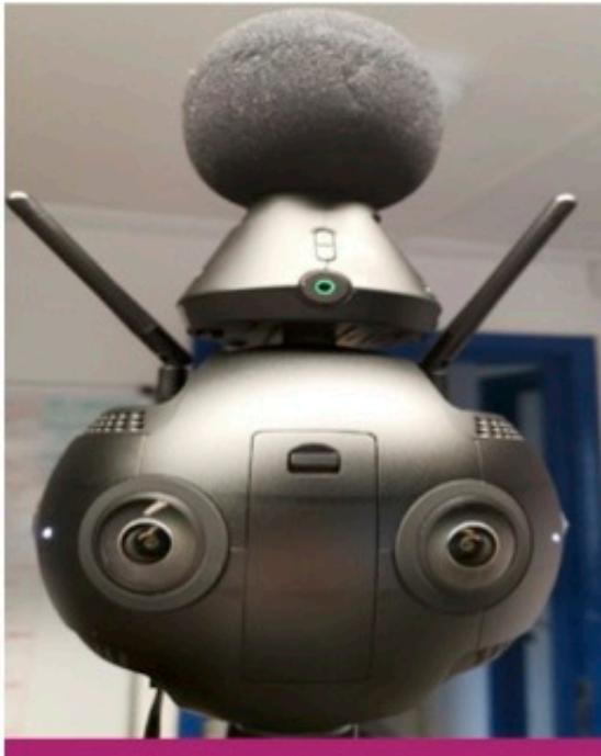
Insta360 Pro 2 with a ZOOM H3-VR audio recorder mounted as a 'hat'
