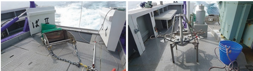
Fig. 22.5 Example of dredge, and grab sampling
